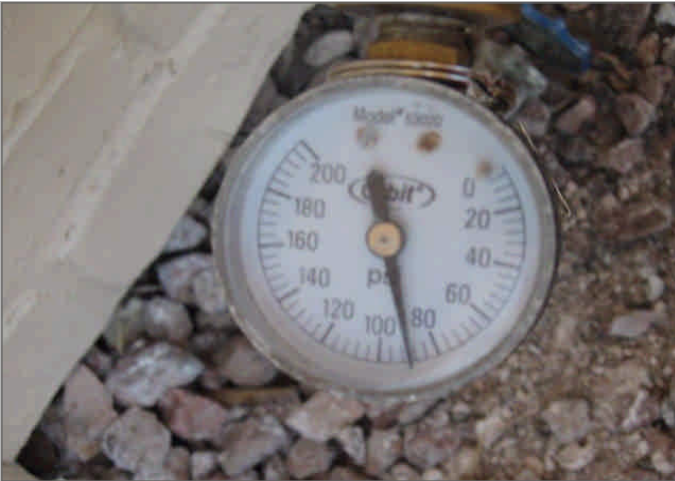
Figure Set 22 - The water pressure was at or over 80 psi
