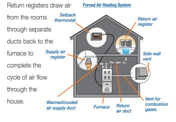
Leaks in forced air distribution systems are often ignored because they normally do not cause any obvious damage, but it is important to avoid/eliminate such leaks. Leaks will affect a distribution system's ability to provide comfort in all areas of the house, and leaks in some parts of the system can result in significant energy loss and/or condensation-related damage which may be hidden from sight.
