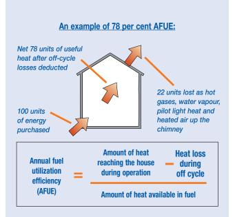
It measures the equipment's performance after it has been running a short while and all components have reached their normal operating temperature. The steadystate efficiency of furnaces and boilers is determined by comparing the amount of heat that's available in the fuel to the amount that is converted into usable heat, but it does not include off-cycle losses.
